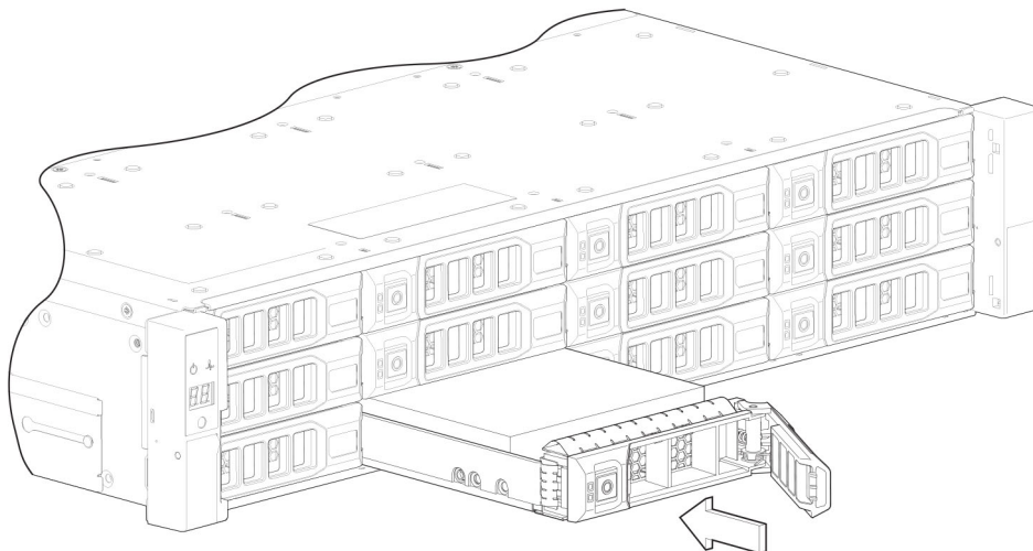
Figure 44. Installing an LFF drive carrier module (1 of 2)
